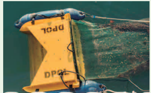
DPOL, a small robot developed in France in 2020 for cleaning water in ports.
